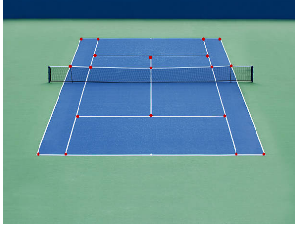
Figure 3.6: Detected and temporally stabilized court keypoints used for homography estimation.
